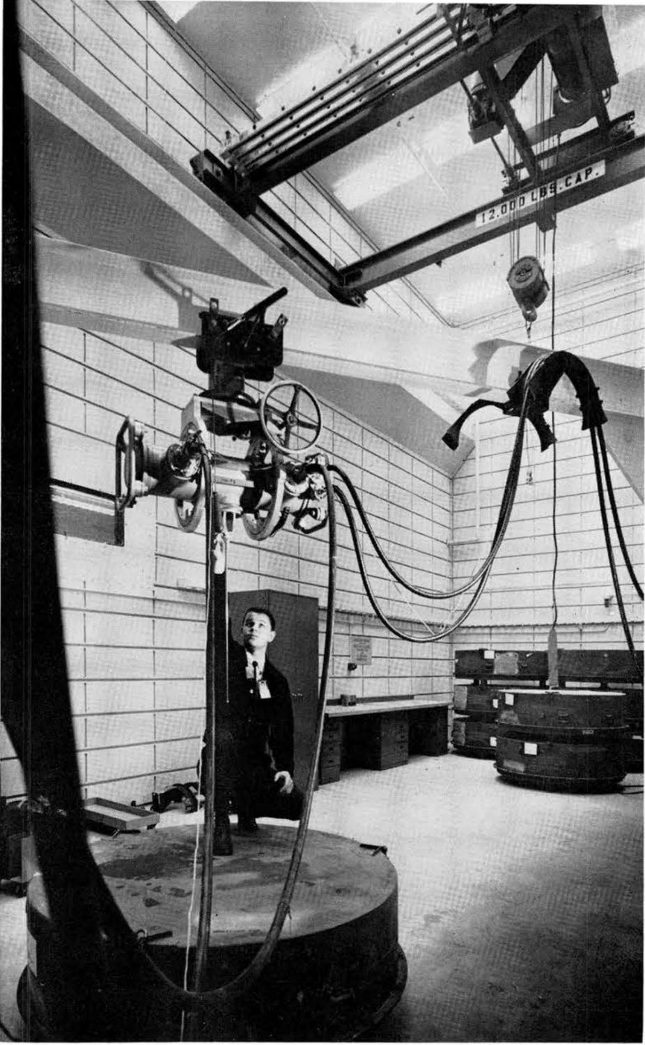
A 300-KV INDUSTRIAL X-RAY UNIT is being positioned by Dennis J. Adkins preparatory to examining a sealed parachute case. The high ceiling and overhead crane provide easy handling for large objects.
