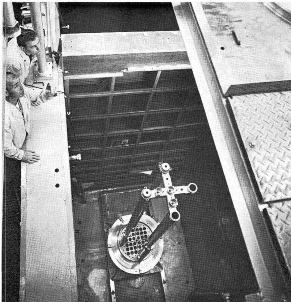
SNARE REACTOR is shown during assembly of the device. It is mounted in a 16-ft. deep pool of water with about 12 ft. of water covering the top of the core. Control rods extend about 10 ft. above the surface of the water. Control instrumentation is located on a balcony above the pool. At left are Roy Tackett of Reactor Division and Louis H. Sanders of Environmental Health Division.
