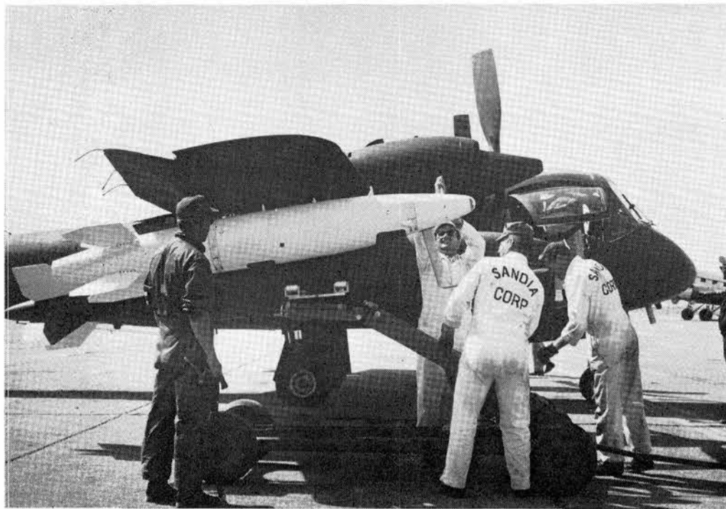
ARMY OV1 MOHAWK stops at Tonopah airport for a quick change of the instrumentation pod. At left is H. W. Pumphrey of Test Operations and Facilities Division, one of the operations project leaders.
