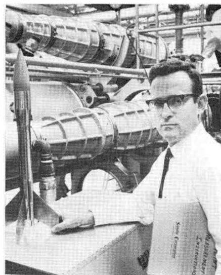
TEST VEHICLE — Jim Reed, Experimental Aerodynamics Division, exhibits a scale model typical of those which are subjected to simulated flight conditions inside the hypersonic wind tunnel at Sandia Laboratory. The tunnel is in the background.
