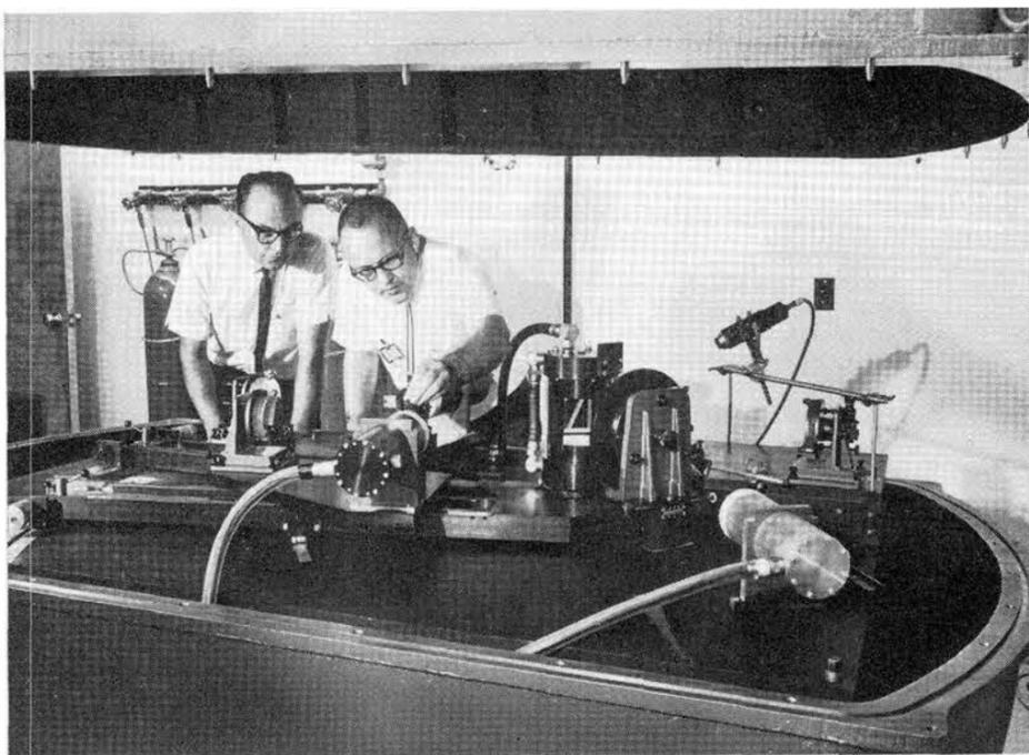
1000-POUND STEEL COVER is lowered when this rapid scan spectrometer is operated in a vacuum to permit rotating mirror (middle right) to reach 1100 revolutions/second. Physicist R. A. Hill (5122) adjusts a detector tube as engineer R. D. Fellerhoff (5141) looks on.
