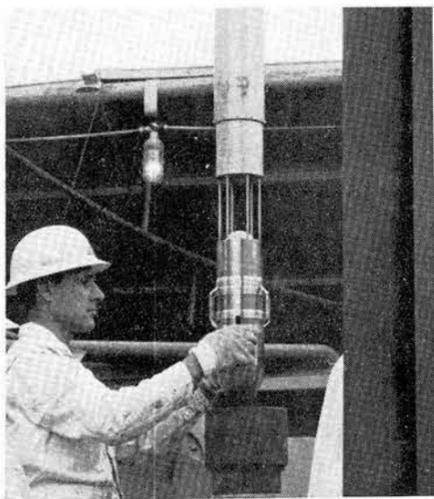
CAVEMAN, an optical surveying instrument developed by Sandia, is positioned above the drill hole on the Project Dribble site by Grover Hughes (7224). The device, by means of a unique optical system, measured the dimensions of the nuclear cavity.
