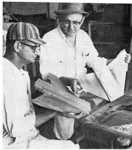
SANDIA'S FOUNDRY made a sand casting from the wooden model—in this case, the wings and part of the fuselage. D. A. Quayle (left) and C. C. Riley (both 4221-2) are checking the almag casting against the pattern.
