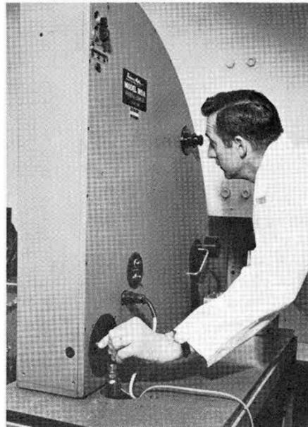
L. E. HEAMES (5134-1) is focusing and aligning framing camera for forthcoming shot. Thick laminated glass in small opening protects camera lens from shrapnel.
