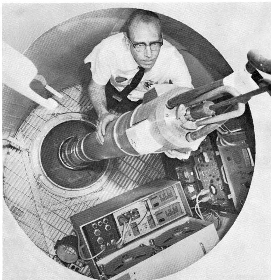
SEISMOMETER PACKAGE is shown as it enters 12-inch-diameter borehole in underground shelter. The USO unit is now 90 feet deep in Alaskan permafrost.
