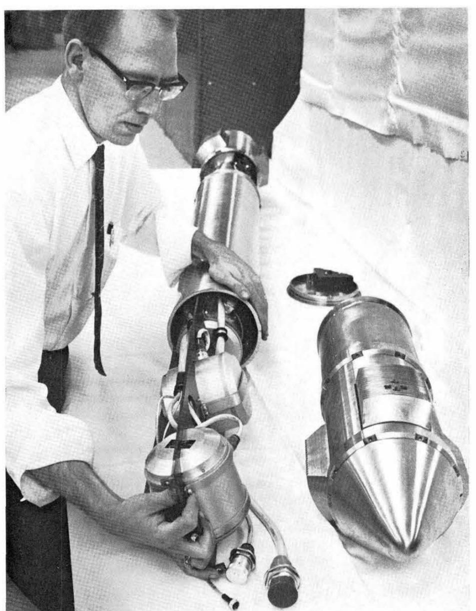
SHORT-PERIOD SEISMOMETER assembly is shown being inserted in a metal cylinder section of the nine-foot-long USO borehole package by Dean Gladow (9233). The long-period seismometer, which is not shown, fits between the nose-cone shaped cap (right foreground) and the forward lock, the section with protruding notched blocks next to the nose cap.
