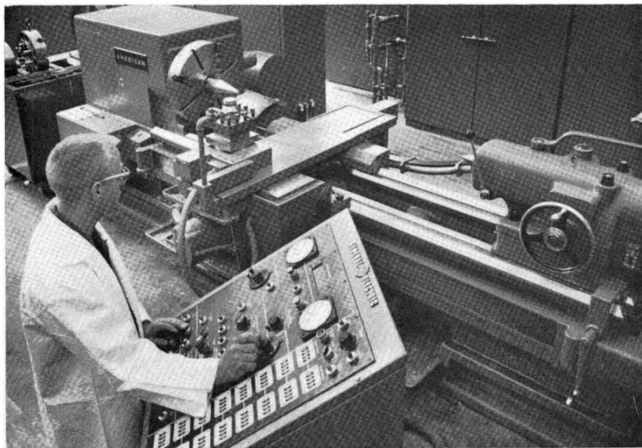
TAPE-CONTROLLED LATHE, recently installed in the Development Shops, is operated by John Malpas (4251-2) using the manual over-ride controls. The new machine has superior production capabilities and unique tooling capabilities.
