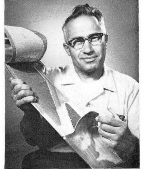
**NICK DELOLLIS** (1133), Sandia's adhesives authority, displays a sample of structural fabrication using aluminum honeycomb bonded with adhesives to thin aluminum walls. Results of a destructive "peel strength" test show that the aluminum failed before the adhesive. Note the honeycomb metal still adhered to upper peeled-back portion.
