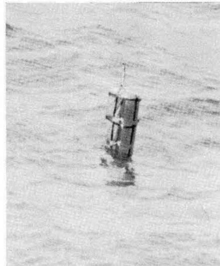
DUAL BAGS with transmitter and antenna float high in the water. Either the ram air bag or the CO<sub>2</sub>-inflated bag is capable of supporting the 150-pound rocket payload, which hangs under the surface.
