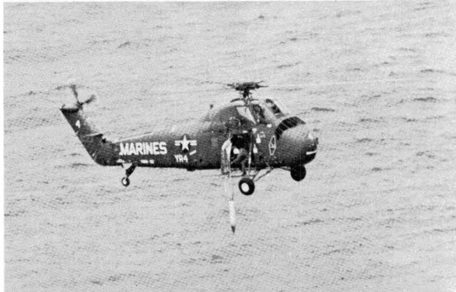
MARINE HELICOPTER fishes a Nitehawk rocket payload out of the ocean near Barking Sands Launch Site in Hawaii. The payload was easily located from the signal produced by the tiny two-ounce transmitter in the Sandia-designed recovery system.
