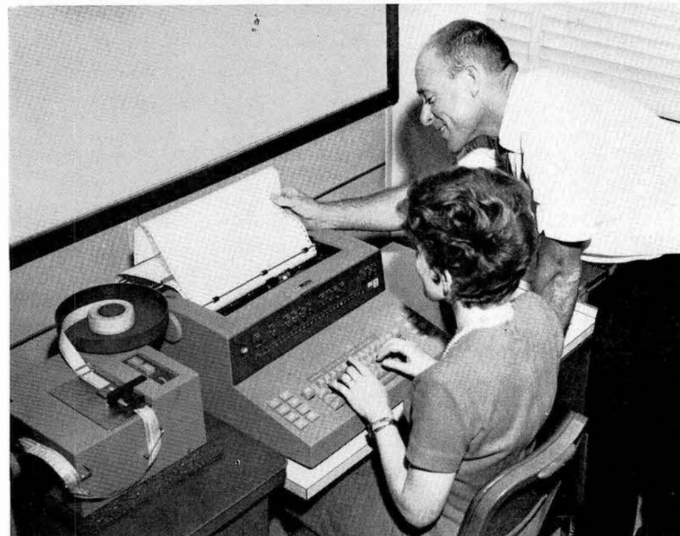
INQUIRY AT A REMOTE STATION is scanned for accuracy by W. J. Harrington, Management Systems and Programming Division 8143. Operator Nancy M. Martin (8253) then releases the request to the central computer where Product Definition Record System (PDRS) information is maintained in computer disk storage files. Requested information appears visually in print out form at the remote inquiry station.
