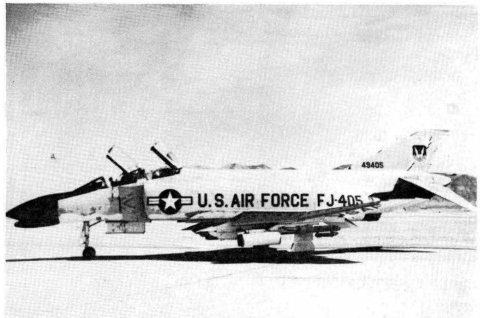
F-4 PHANTOM, the Air Force's fastest and highest flying fighter-bomber now in operational use, is one type of aircraft participating in the current JTF-2 flight tests in Arkansas. It is a two-engine, two-man, all-weather weapon system now being used in Southeast Asia.
