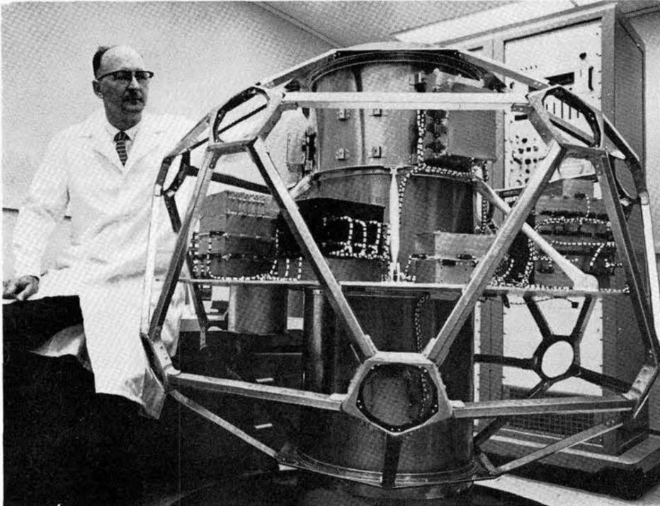
VELA SATELLITE MOCKUP was used to check the installation of the Sandia logics systems before the components were shipped to California. Shown with the 26-sided model is J. C. Rehberg of Satellite Systems Division II, 9234.
