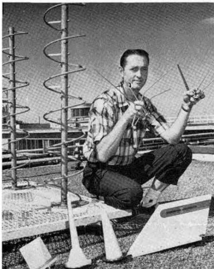
VARIOUS ANTENNA SHAPES are displayed by Robert A. Leighninger (1424) on the roof of Bldg. 802. Bob is shown holding a nose probe and a selection of both angled and straight whip antennas. Helix antennas are on the left with three plastic covered antennas in the lower left foreground. A fin-mounted dipole is in the lower right foreground.
