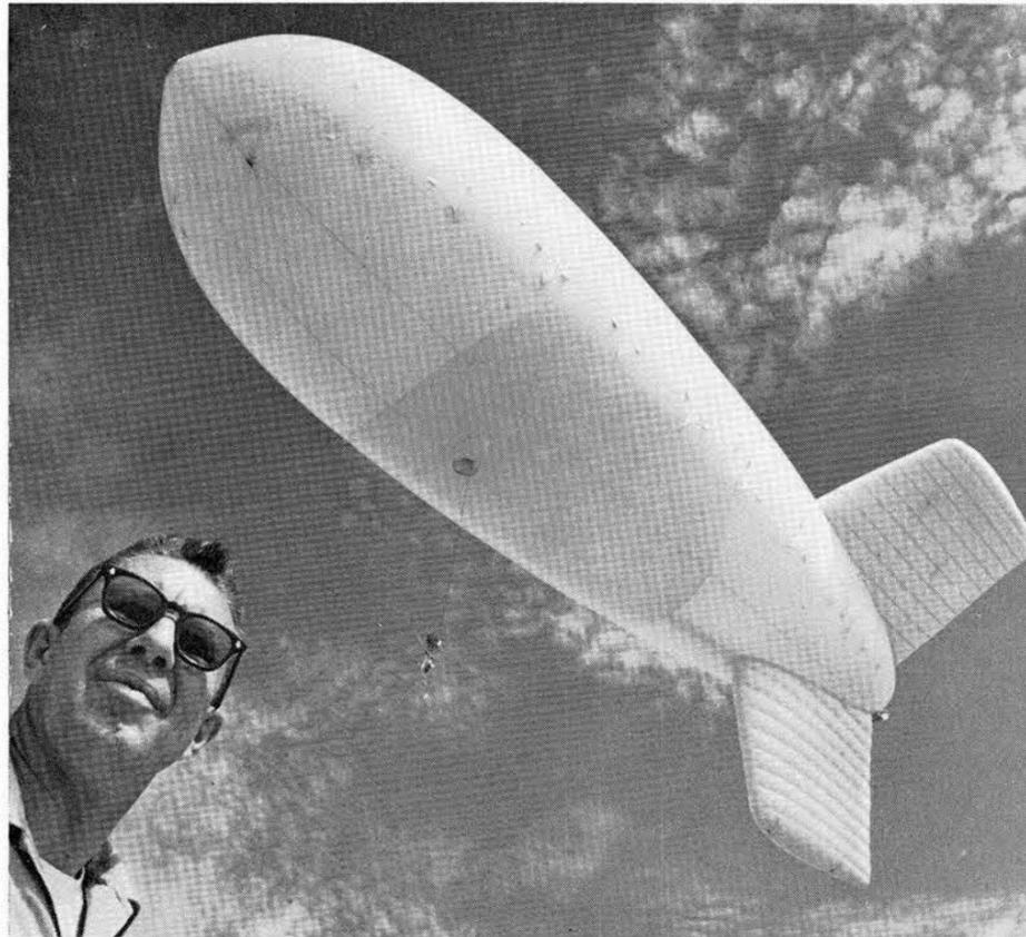
SKY-HOOK—New prototype balloon flies above the head of designer H. G. Laursen (7242) in Coyote Test Field. The 72-foot-long balloon will support strings of air blast pressure gages.
