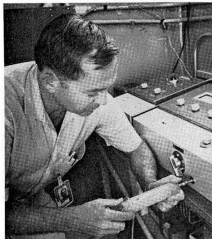
LIAL BREWER (3311) checks the gas chromatograph instrument which enables remote sampling and analysis of tunnel gases following detonation.
