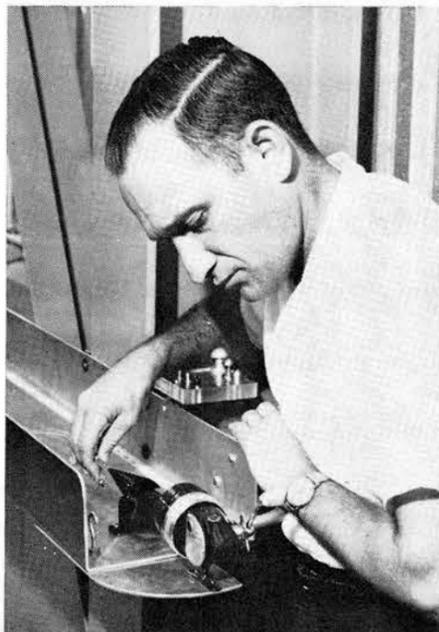
L. F. DANIEL (8223-3) demonstrates pneumatic sleeving aid he designed. The device has reduced the fabrication time of multi-conductor cables to a fraction of the time required under the old method.
