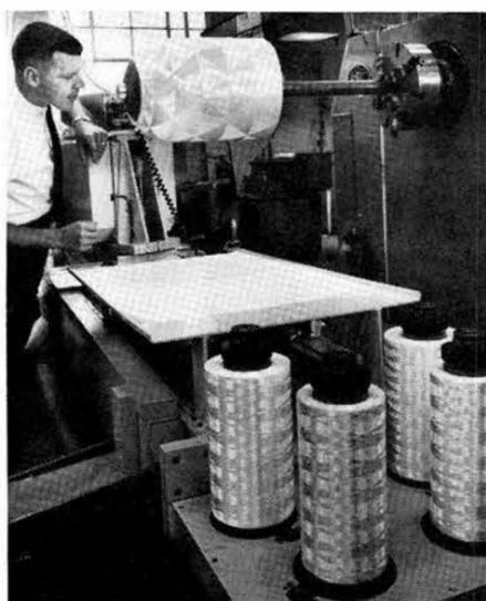
FILAMENT WINDING, part of a process which produces tough-as-steel parts from glass threads and coatings of plastic, will be demonstrated in Sandia's Plastic Shops, Bldg. 834, during Family Day tomorrow.
