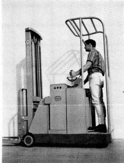
BEFORE MODIFICATION, A FORKLIFT SAFETY COVER offered little protection for operator Bob Tirnetta's (8245-3) head and back (left picture). After modification, the new cover and platform (right) provide maximum protection for Bob.
