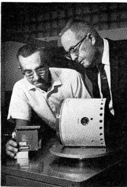
AIR BEARING DEVICE, which measures moment of inertia almost independent of the test object's weight, is positioned by designer C. E. Miller (left) while his supervisor, R. N. Browne (7214), follows the operation.
