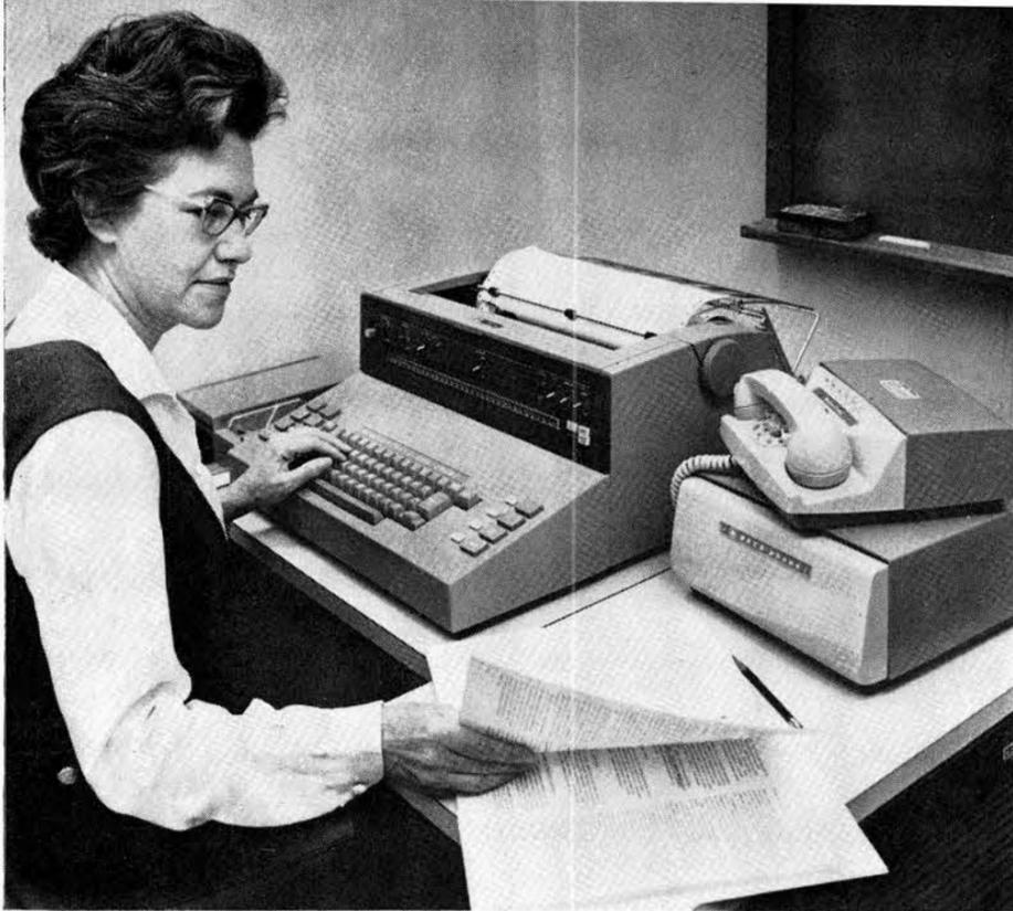
REMOTE COMPUTING CONSOLE in Bldg. 836 is linked to a computer in Los Angeles by long distance telephone lines. Elizabeth L. Frost (2153) demonstrates how the time-sharing system makes it possible to write, edit, compile, execute, and debug a program on the printer console.
