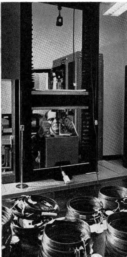
FRANK BATCHELOR prepares a filament wound specimen for static testing. The universal test machine will load the hoop in compression and the resulting measurements will indicate the material's strength. In the foreground are more samples awaiting test.
