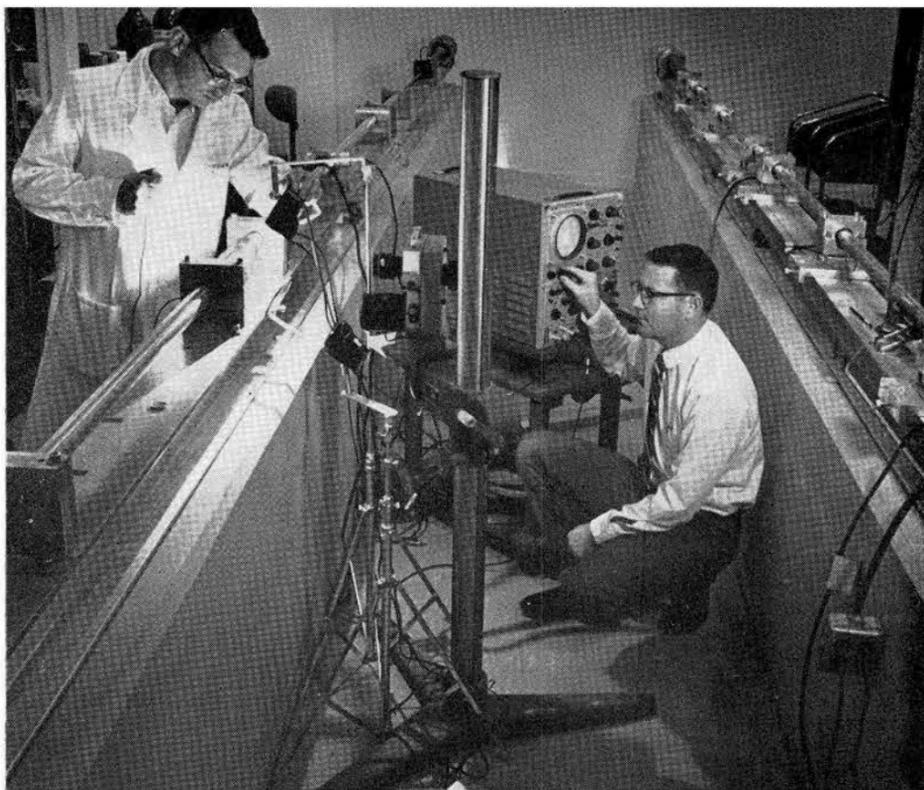
HIGH STRAIN RATE TEST of a plastic material is prepared by E. R. Dunaway (left) and O. L. Burchett on the Hopkinson pressure bar device. High speed photographic coverage will yield a visual record plus superimposed oscilloscope data on the film. Test will show the strain rate sensitivity and the failure mode of the material.
