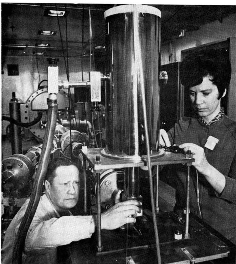
PHYSICIST RUTH WHAN (5211) attaches thermocouple wires to monitor sample temperatures during irradiation on the Van de Graaff accelerator while R. S. Neiman hooks up an electrical connection to monitor radiation levels.
