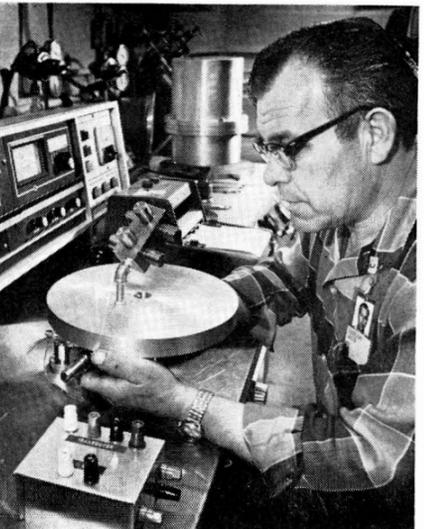
JAKE BARRERAS readies a test jig prior to a leak detection test. The test will determine the number of extraneous molecules collecting in a sealed component resulting from materials "outgassing."
