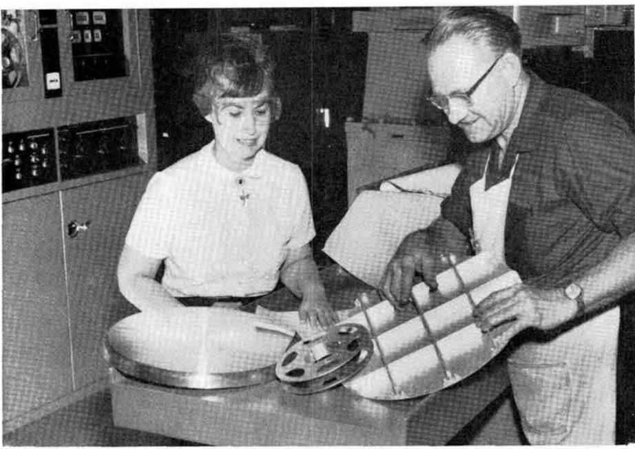
REBUILT MILLING MACHINE gives Livermore Model Shop capability of making three-dimensional parts by numeric control. Secretary Vivian Lenz observes while Model and Instruments Maker G. H. Brockmoller (both 8223) shows the completed grid the machine made from a smooth aluminum disc. Converted mill and updated solid-state control panel can now fabricate parts 10 x 20 x 30 inches.
