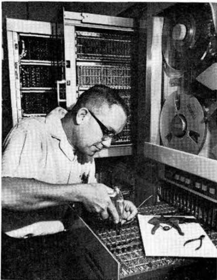
R. L. SHAUM (7222) is modifying one of several hundred transistor circuits in this card drawer of the Tonopah-bound data processor. The racks behind him each contain some 200 printed circuitry boards.
