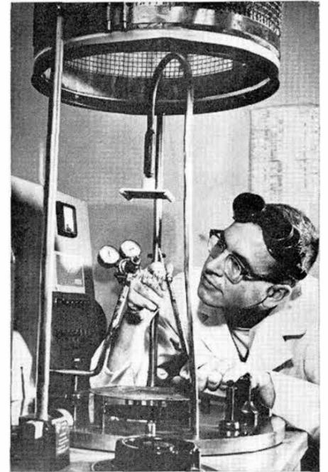
A PATENT has been issued for this apparatus, invented by D. M. Mattox (1123), which makes possible ion plating of numerous metals which could not be coated by conventional techniques.
