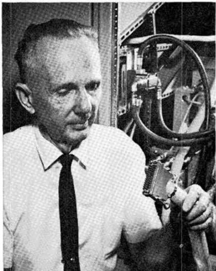
FLUIDIC CONNECTOR was one of the innovations Max Bleakney (2451) created for new fluidic production tester. Fifty air tubes are handled as a single cable, fit into a modified electric connector.
