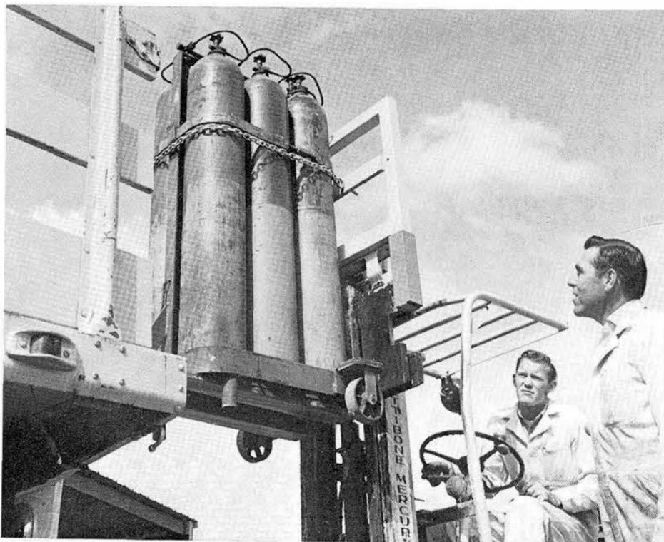
MODIFIED FORKLIFT holds the load secure while John Tootle, operating forklift, and Stan Serpa (both 8245-3) unload compressed gas cylinders. Design of the removable metal frame and its chain by John and Stan reduces handling hazards for six-pack units.
