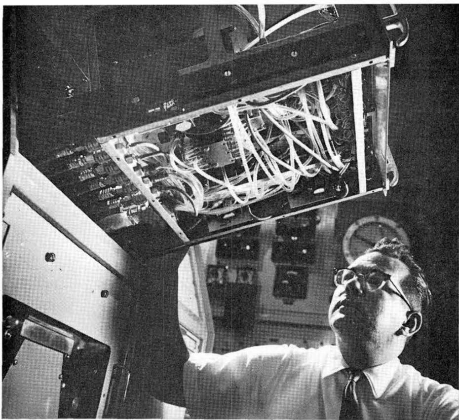
FLUIDICS CONTROL PANEL, which controls automated testing of nuclear weapons in final assembly stages, is inspected by Ron Oelsner. Previous testers for final checking were manually operated due to limits on amount of electric power that could be used.
