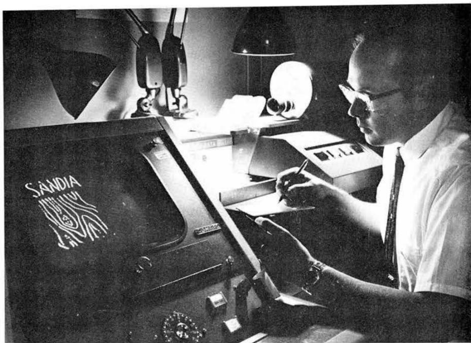
CONTOUR LINES of a terrain map and a handwritten "Sandia" are projected on the Sandia Image Digitizer's monitor screen as R. K. Cover (2565) notes some operations. The Sandia-developed system converts illustrations, such as graphs and waveforms, to digits for computer processing.
