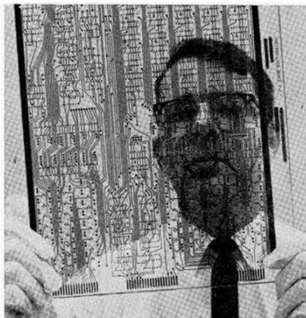
FINISHED PRODUCT of the Precision Numerically Controlled Drafting System, in this case a master drawing for a printed circuit, is displayed by A. D. Bridegam, 2211-5 supervisor. The system can also produce precision graphics for tiny micro-circuits and other applications.
