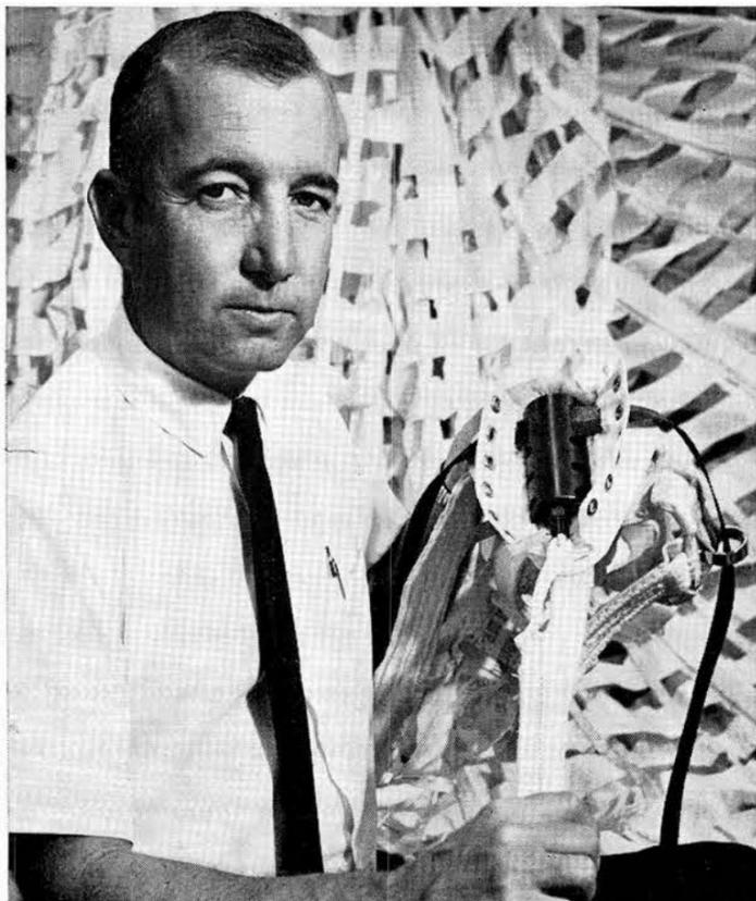
REEFING LINE CUTTER on a 20-foot diameter ribbon parachute is displayed by James P. Gallagher (9323), inventor of the device.
