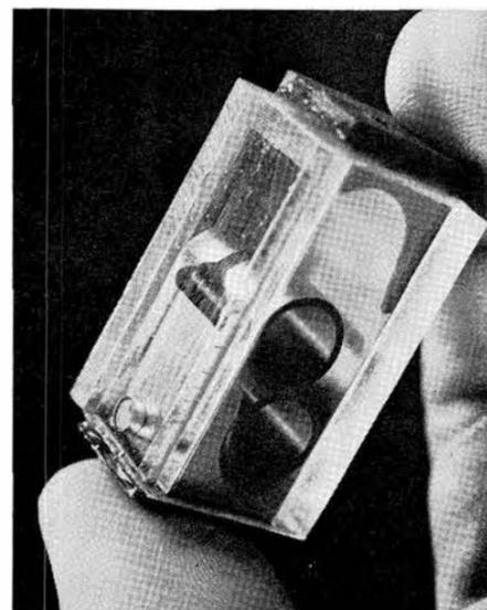
TYPICAL ROLAMITE configuration is used here as a gravity switch. The cutout in the band around the rollers helps introduce a force into the roller cluster equal to a specified gravity, such as 12 G's. When an accelerating vehicle reaches this G-level, the cluster breaks away, snaps to the right, and closes (or opens) an electrical circuit.
