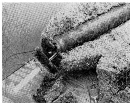
FUEL CONTAINER tested in a mixture of Bentonite, Ottawa sand and feldspar melted near the top. Half of the sintered soil mass which completely surrounded the container has been removed to show the condition of the container. The mass was created by the soil melting and sintering under high temperatures.
