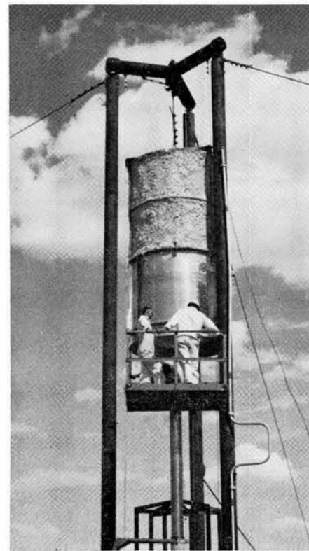
DROP TEST of 25,000 pounds of liquid oxygen and RP-1 (kerosene) is readied by range personnel at Edwards Air Force Base. Coating around upper portion of tank lowers boil-off rate of liquid oxygen. Pie-shaped cutter on stilts below the tank ruptures the containers during the drop and a small explosive charge ignites the mixture.
