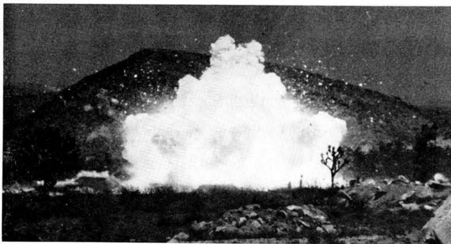
FIREBALL CREATED by 100,000 pounds of liquid hydrogen exploding during a test simulating a failure of Centaur upper stage.
