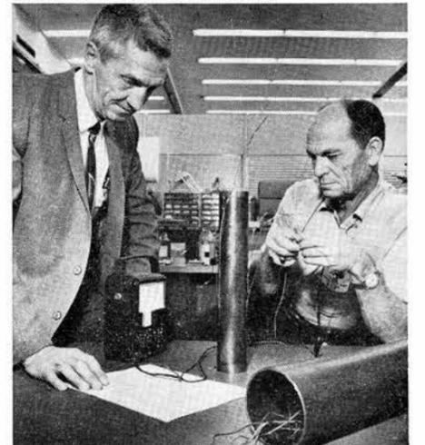
HEAT TRANSFER SPECIMENS are checked at the Laboratory by Frank D. Kite (9312), left, and O. A. Phelps (7215). The instrument is used in Project Pyro tests to gather heat transfer data for aerospace nuclear safety program.
