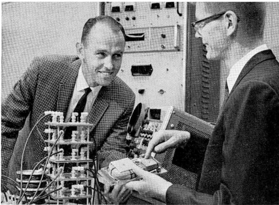
INVENTORS Elmer E. Smith (8151), left, and former Sandian Hartley J. (Nick) Jensen discuss two versions of their electronic device which measures the time interval between a number of electrical pulses to an accuracy of  $\pm$  one nanosecond. The laboratory apparatus in front of Elmer can store five electrical pulses.
