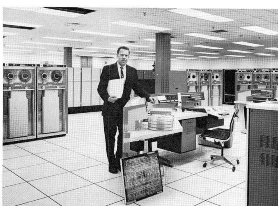
PORTION OF UNIVAC 1108-II multi-processing computer equipment in the new addition to Bldg. 880 surrounds R. M. Campbell (9411-4). Additional UNIVAC equipment is hidden from view in the background.
