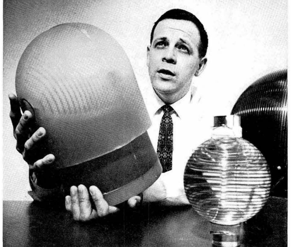
SANDIA-DEVELOPED SPHERICAL ANTENNA used in a recent test is held by T. W. H. Caffey (7211), who designed the telemetry system. The antenna is potted in plastic to protect it from environmental conditions. The other spherical antennas shown in the picture are developmental models.
