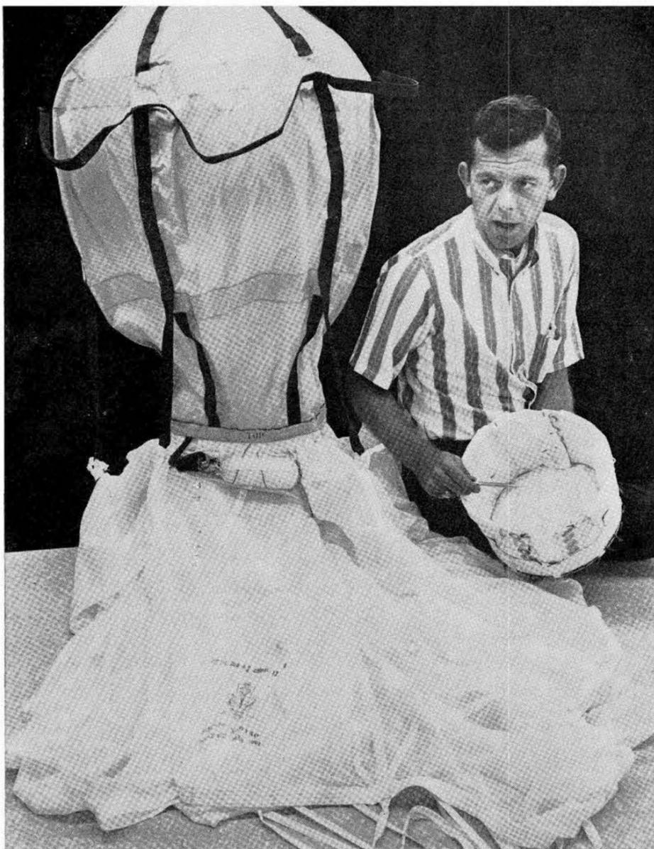
HOLDING THE BAG that houses the new recovery system on rocket flights, Don Johnson (9324) explains packing procedures. The ram-air bag is shown suspended in the center of the picture with the eight-foot parachute draped on the table below. The seam between the two conceals the hole through which the air passes to inflate the bag. The dark colored, looped strap around the bag is a recovery line.
