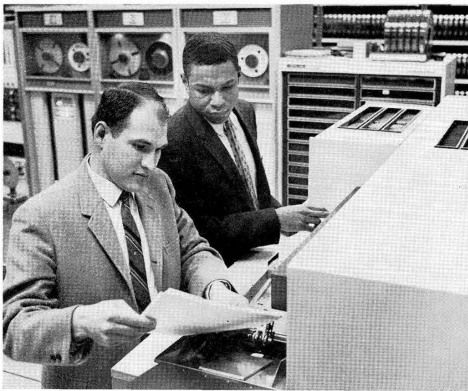
PAGES OF TEXT are fed into the page reader of Sandia's new optical scanning system by A. A. Key (9427), left, as A. L. Hardeman (9426) checks the control buttons.
