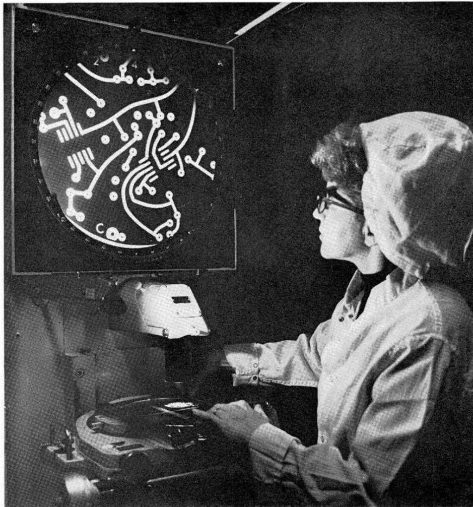
OPTICAL COMPARATOR with 100 magnification is used by Dorcas Gabaldon (4233-3) to check for possible breaks or flaws in circuit paths.
