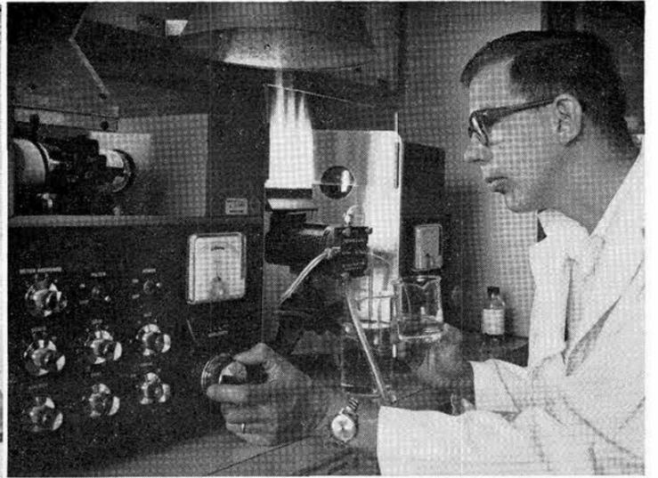
ATOMIC ABSORPTION SPECTROPHOTOMETER is operated by J. P. Grillo (3311) to analyze the content of a particular metal in a sample. Emission tube (upper left corner) radiates characteristic lines of the particular element under study and provides a basis for comparison. Through use of this instrument analyses that previously required days of lab work can be performed in 10 minutes.
