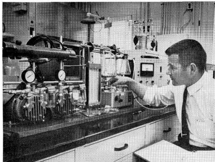
DYNAMIC SOLVENT vapor generator is being used by D. R. Parker (3311) to calibrate a halide meter for accurate readings in the field. The generator produces standard concentrations of gases or vapor which can check the accuracy of air sampling equipment used by industrial hygienist.
