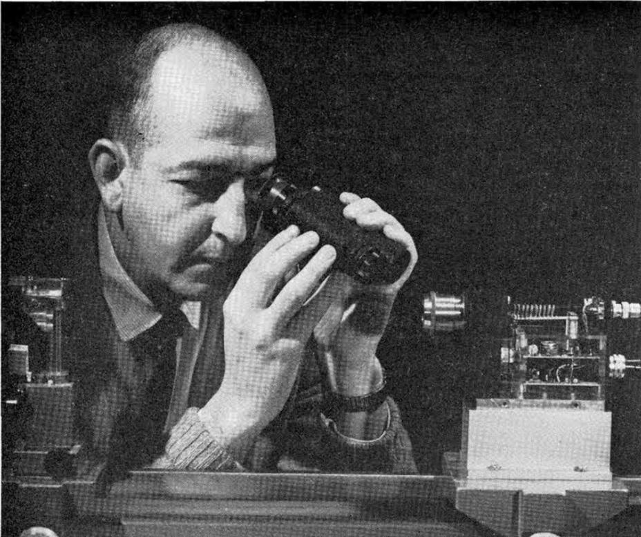
LASER LIGHT SOURCE focus is checked by Bob Miller (8119) with an electronic image converter (which is similar to the Army's "snooper scope"). Designed and developed by former-Sandian J. W. Stull and Bob, the small portable laser (right) is used to test photodiode operation (left) in intense light. It produces a fast-rise, intense, repeatable source of light for testing fast response photodiodes at infra-red frequencies.
