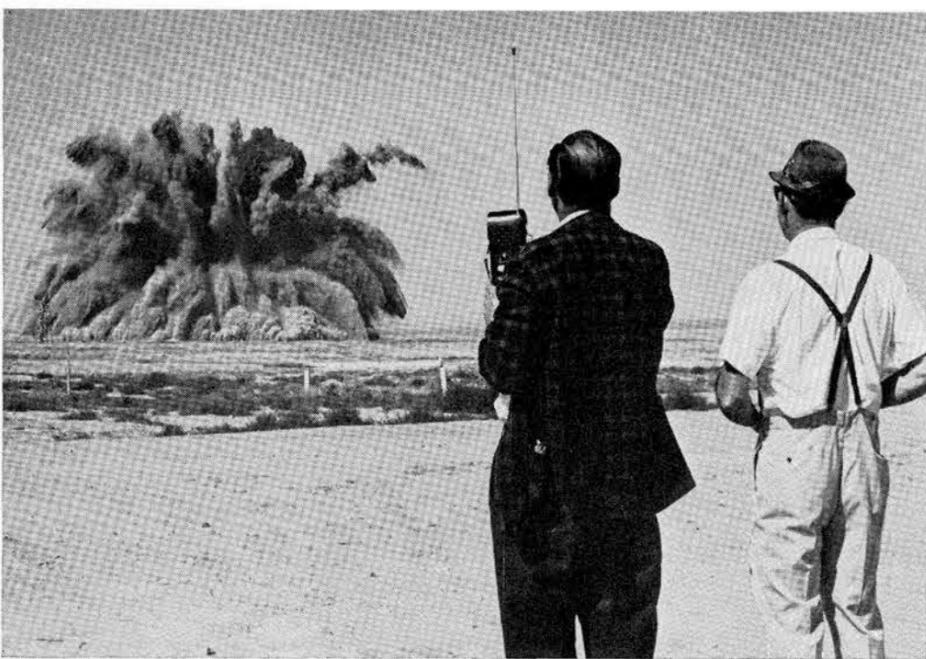
DETONATION of a buried charge of 30,500 pounds of conventional high explosives in Coyote Canyon Test Field created a dust cloud and a crater about 30 feet deep and 105 feet in diameter. The blast was part of a Plowshare experiment to study air-blast geometry. At left is Virgil Harris (9133), Field Test project engineer, with L. J. Vortman (7111), scientific advisor for the project.
