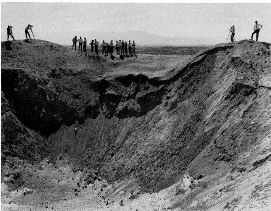
MORE THAN 7200 tons of earth were tossed out of this 105-foot diameter crater created by the detonation of a buried charge of 30,500 pounds of high explosives. The experiment, primarily conducted to study air-blast geometry, also contributed to a knowledge of cratering mechanics. The photographers are shooting film for local television.
