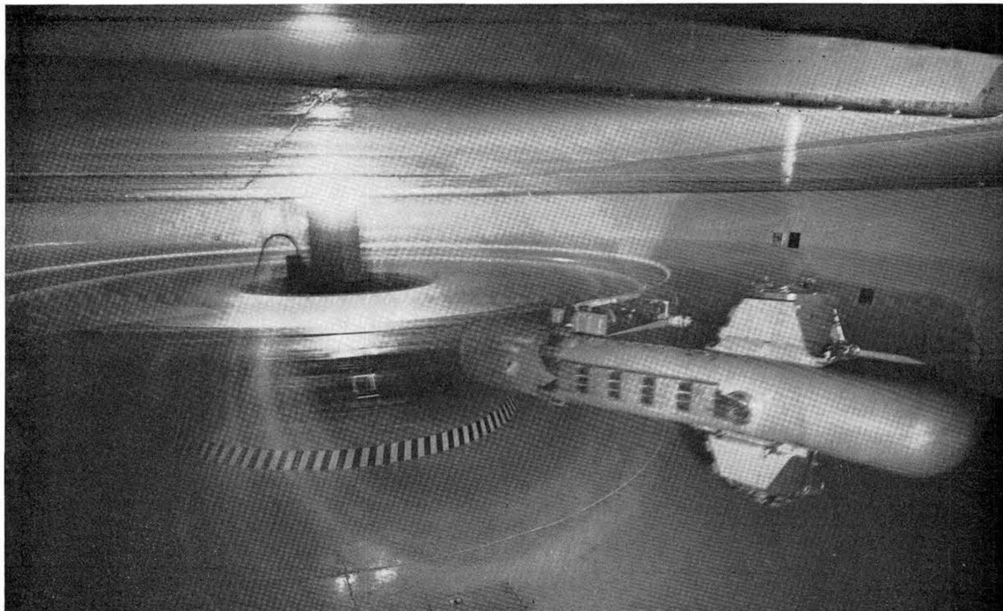
MASSIVE 30-TON ARM of Sandia's underground centrifuge now has twin shakers mounted on one end to provide acceleration and vibration environments simultaneously. The forces duplicate the conditions
