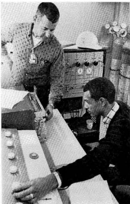
GAS SAMPLES from inside the test tunnel are piped to this gas chromatograph for analysis by Don Parker (3311), left, and Billy Smith, REECO health physicist.
