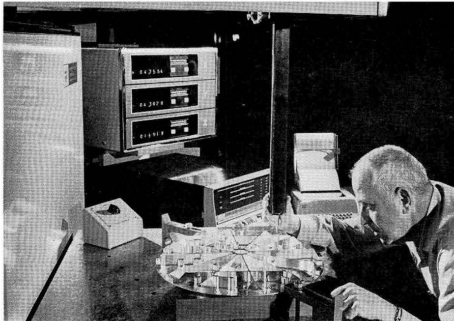
NEW THREE-COORDINATE MEASURING MACHINE is used by John Barnhouse (8226) to check the hole configurations in mounting pads. Recently operational, the equipment is accurate to  $\pm .0005$  of an inch and prints inspection reports automatically.
