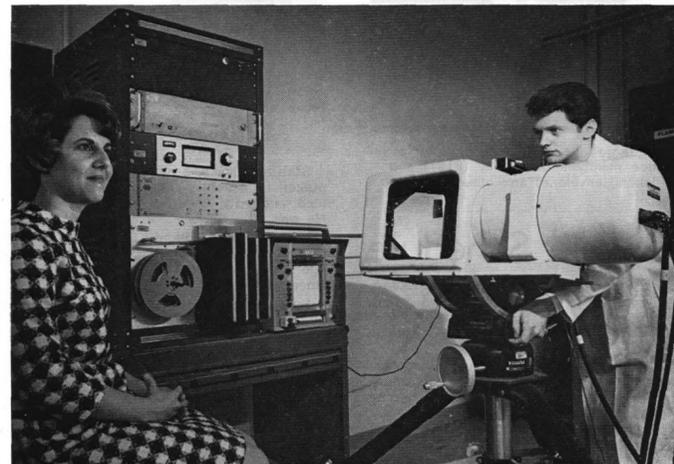
JERRY STOKER demonstrates capability of an infrared scanning camera to perform temperature analysis by training its scanning mirror on the face of Diane Cleveland (3126). The camera can detect minute temperature differences, which may indicate defects, over a range from -170° to 250° C. It is not dependent on external sources of illumination, but responds only to the infrared energy radiated by all objects.
