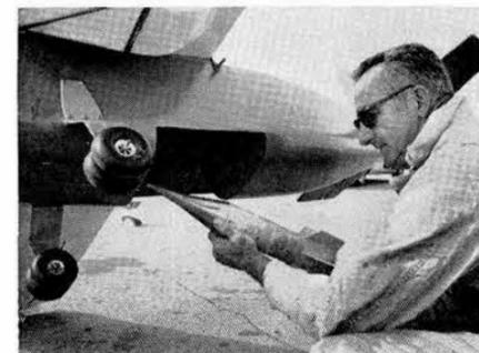
TERRADYNAMIC test unit is loaded into the bomb bay of the Beast by Chad Miller (7214). Release mechanism for the drop is controlled by the "pilot" using a radio transmitter.
