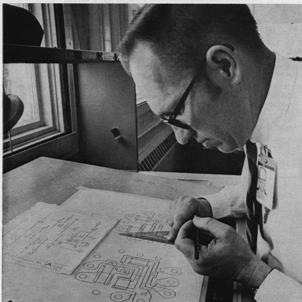
FIRST STEP of a simple process for obtaining a highly sophisticated component. The initial circuit layout is done on a 20:1 scale and reduced photographically. Dick Knutson (2633) translates a circuit schematic into a microcircuit layout.
