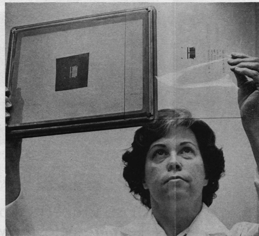
SILK SCREEN is checked against original mask by Ruth Wright (2633). In this case, a fine weave stainless steel mesh is used instead of silk.
