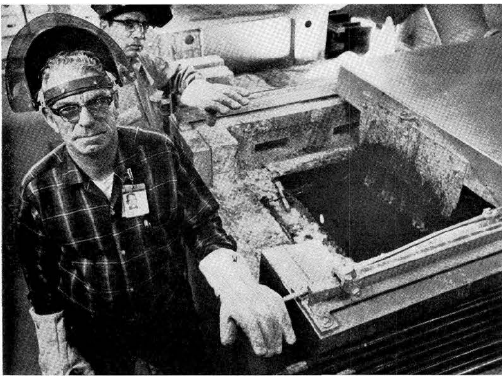
HOTSTUFF —Silas Shane (4512), left, is the newest member of the Wise Owl Club of America. Silas escaped blindness by wearing a face shield when changing a heavy heating element in this hot salt bath. The element broke while being hoisted out of the tank and splashed the 1400° F solution onto Silas' face shield. He suffered only minor burns. Eusebio Montano, in background, was standing just inches away but was uninjured.
