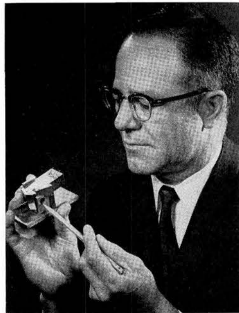
"SUPER-SAFE" SWITCH, invented by Charles Sandoval (2325), has shock and vibration-proof features. Solenoid-operated device is actuated by an electrical signal.
