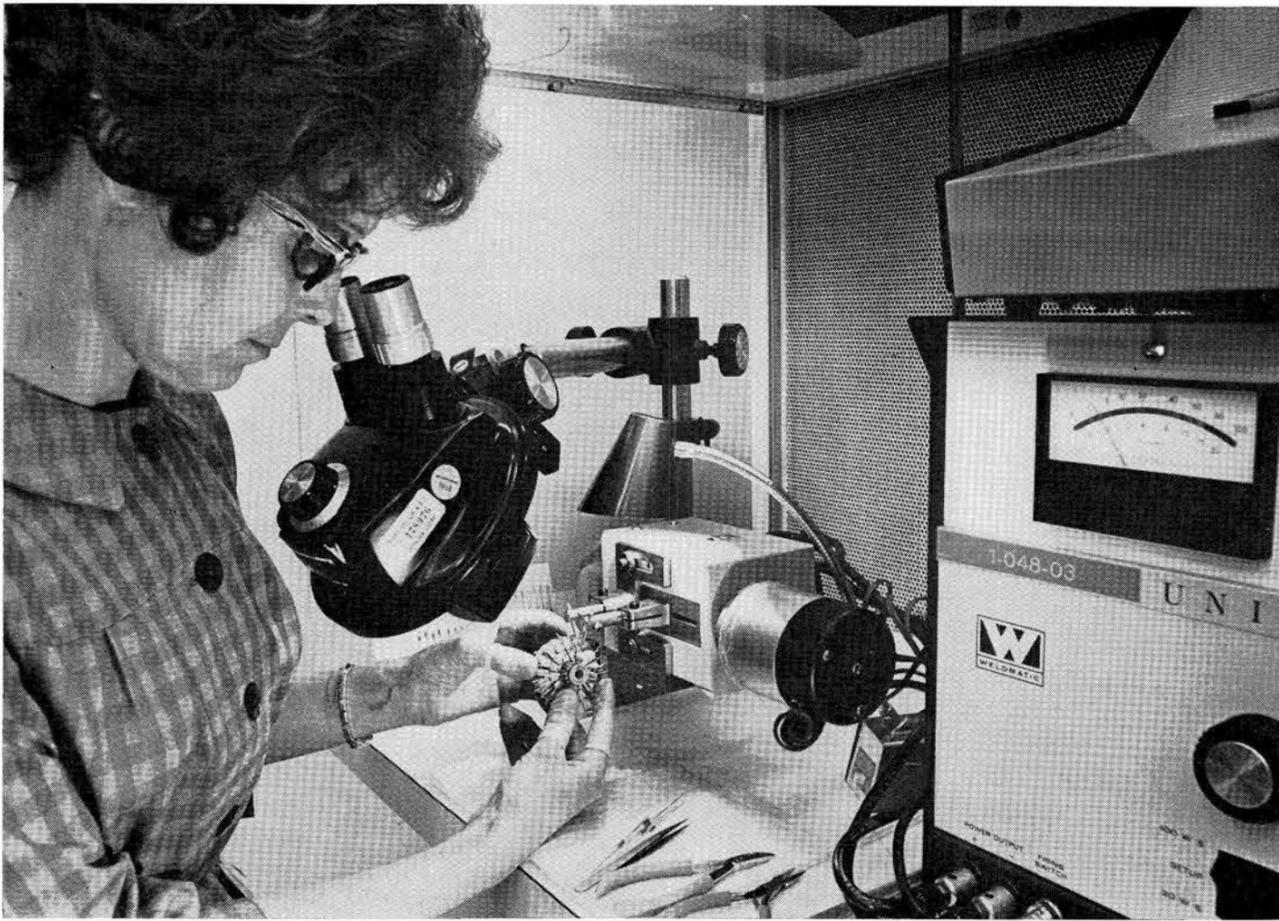
**RESISTANCE-TYPE WELDING** is used by Delores Smith as she works on a Marx generator. Each device has 135 welds and differences in combin-
