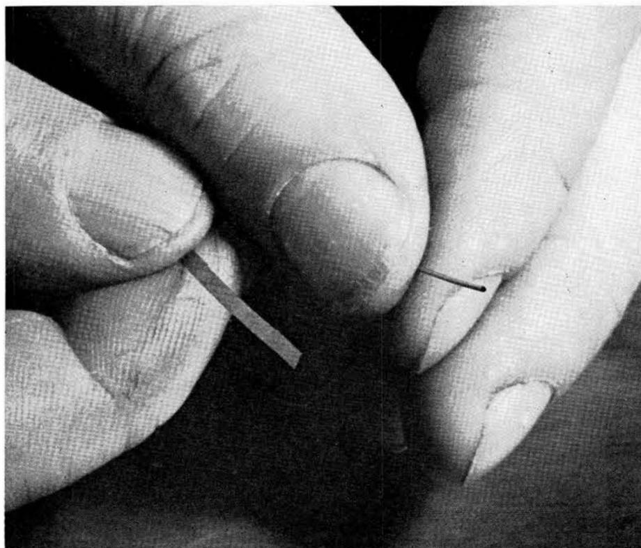
**TAKE A PIECE OF METAL** (in this case, rhenium) roughly the width and thickness of the opening tab on a pack of gum. The problem is how to roll the strip into a three-inch tube and weld the lengthwise seam.
