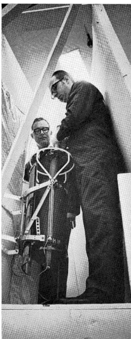
PROTECTIVE GRAPHITE CASK, mounted outside the LM, will hold the SNAP-27 fuel capsule while traveling through space. Al Stephenson, right, and Jim Leonard practice installing the fuel and securing the dome on the cask. Loading the fuel is performed at T minus 15 hours in the Apollo countdown procedures.
