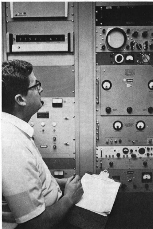
CESIUM BEAM frequency standard is the "atomic clock" in Timers Division 2326. Cesium tube is in the bottom panel. Joe Losinski adjusts equipment, accurate to a few parts in  $10^{11}$ . An "atomic second" is defined as 9,192,631,770 vibrations of a specific transition of the cesium atom.
