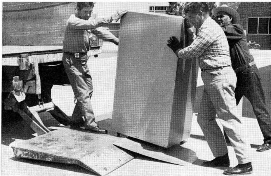
RUDY LUCERO, left, demonstrates how an aluminum plate attached directly to the power tail gate of the devily truck simplifies the loading job. The heavy safe can be rolled directly onto the gate, impossible to do without the plate. It saves about four minutes per job. At right are Manuel Sanchez and Fidel Gonzales.
