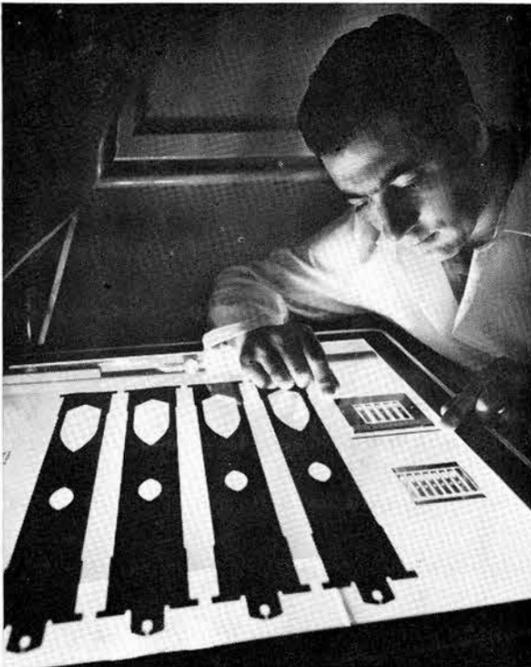
ROLAMITE BANDS are produced from 10-times oversize drawing prepared by Precision Graphics Section 7653-1. The large negatives are photographically reduced to size by Printed Circuitry Lab Section 4221-1 and then the image is transferred to metal and etched in the Rolamite Lab. Tom Cleveland (4222-3) compares negatives with finished set of metal bands.
