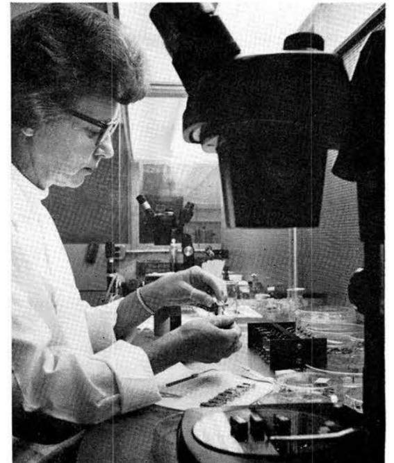
VERNA CLARK (4222-3) assembles rolamite switches at a clean bench location in the Rolamite Lab. A complete rolamite fabrication technology has been developed and transferred to outside suppliers for production of rolamite switches.
