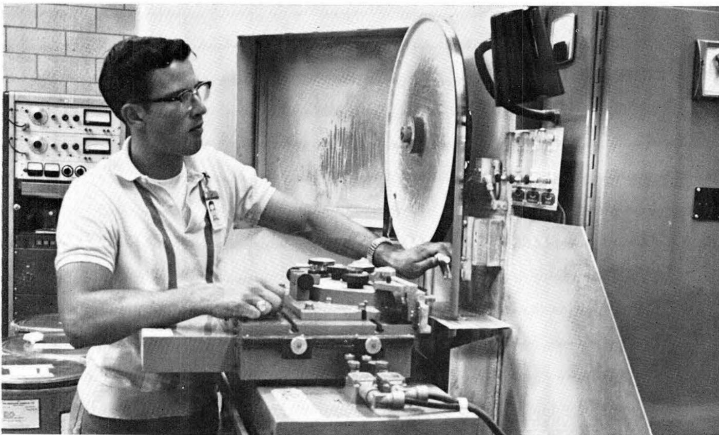
24-CARAT cuts are assured with this diamond band saw in Ceramics Lab. One of two such recently-acquired instruments, the saw can make repeated cuts accurate to within two thousandths of an inch (.0002"). Ceramics, quartz glass, carbon, or any other extremely hard material can be cut with ease by the 118-inch long diamond-coated band. A unique feature of
