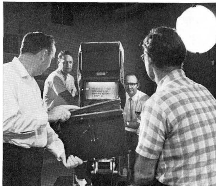
TELEPROMPTER, also called the idiot board, is part of well-equipped studio. The device is mounted on an Auricon 1200, a 16-mm single system camera.
