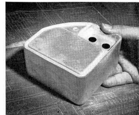
UNIQUE CAPABILITY of the electron beam welder in the Welding Laboratory is evident in the weld on this electronic component. Most electron beam machines will weld only straight lines or circles, but the Sandia unit will weld any contour of a single plane. Roman Heuer (7512) drew up the specifications for the unit, the only one of its kind.
