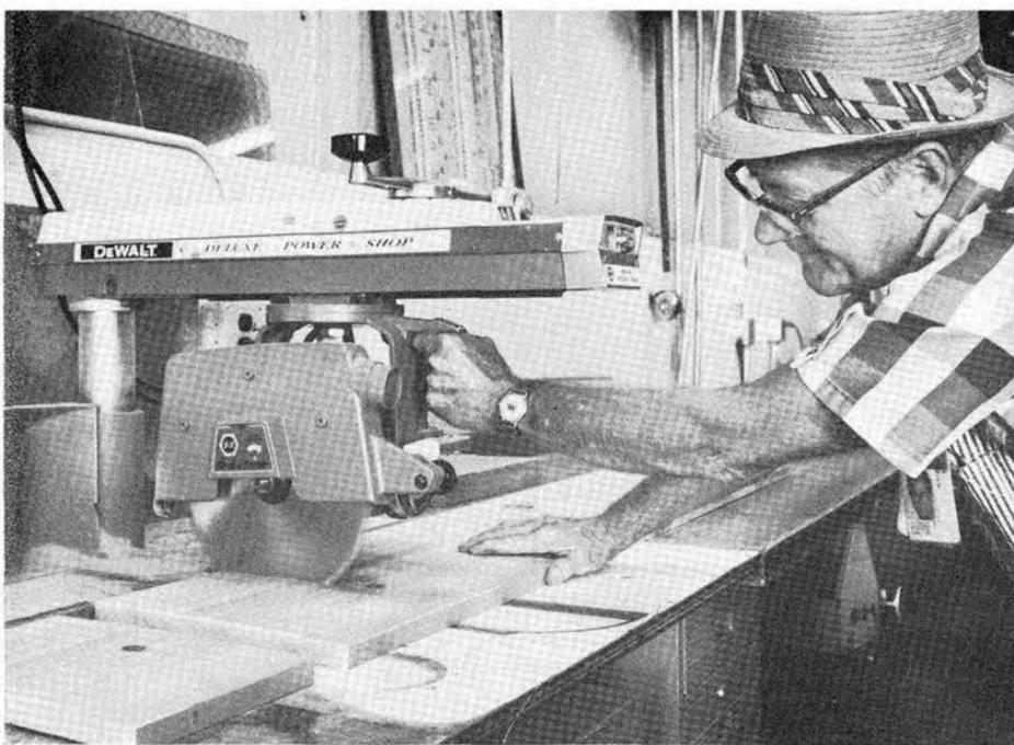
FINGERS cut easier than boards which is why Doomas Easton (4512) keeps his out of the way when using a power saw. Doomas urges power equipment operators to read directions furnished by the manufacturer for proper — and safe — techniques.
