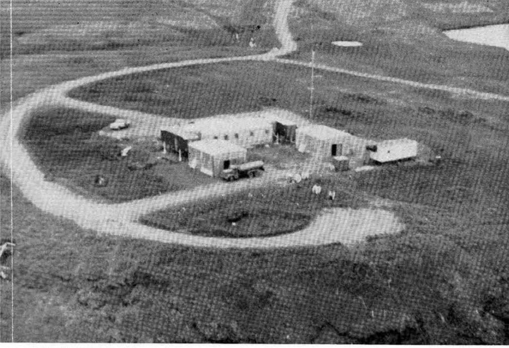
**AERIAL VIEW** of Sandia's recording trailer park shows the post perched on the tundra above rocky shore line. Both hard wire and RF telemetry link was used in recording data from detonation.
