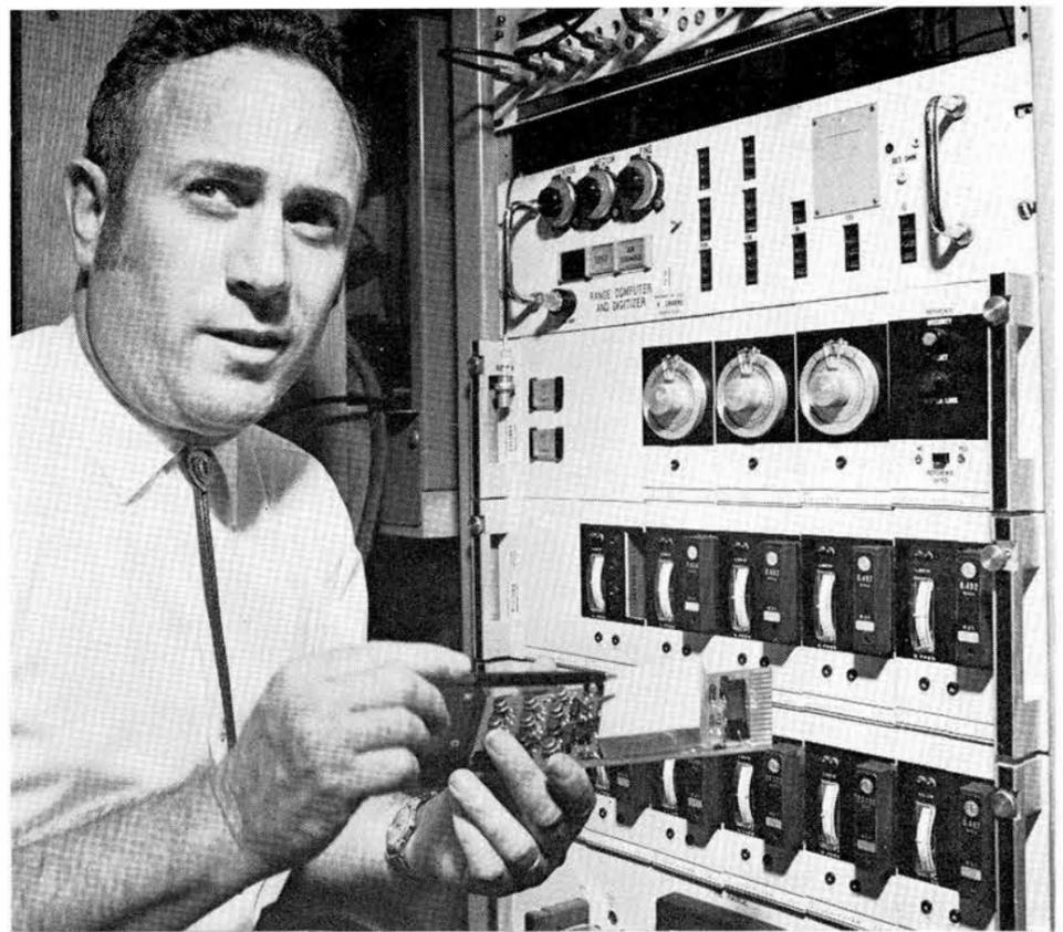
SPACE SAVER—These two banks of electronic tracking filters take the place of the nine racks of equipment previously required to obtain distance data during rocket tests. The array of filters was designed by Murray Silverman (9222) and will yield data from as many as 32 rockets.
