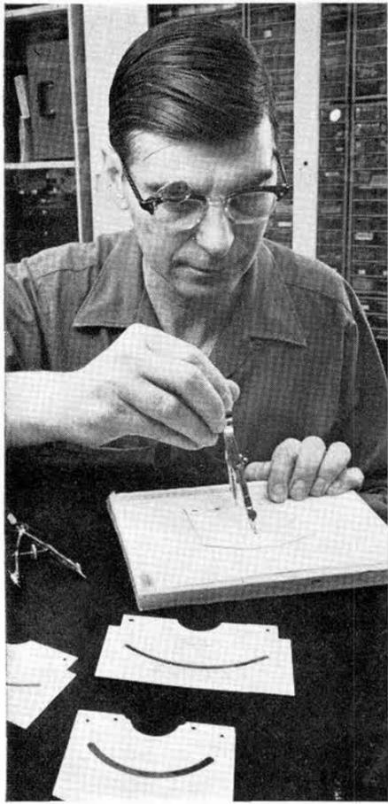
RESCALING and refinishing meter dials is one of the jobs carried out by Kent Johnson.
