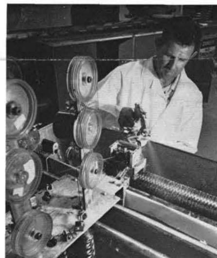
RON GOLDING (5312) operates a small filament-winding machine. Pure carbon filament is being wound around a mandrel while Ron sprays the piece with a thin adhesive.
