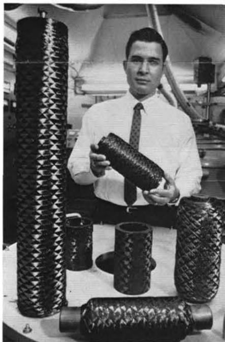
DAVE THEIS (5312) displays a variety of filament-wound carbon/carbon shapes produced in Sandia's Carbon Process Laboratory. The material will undergo extensive laboratory testing.
