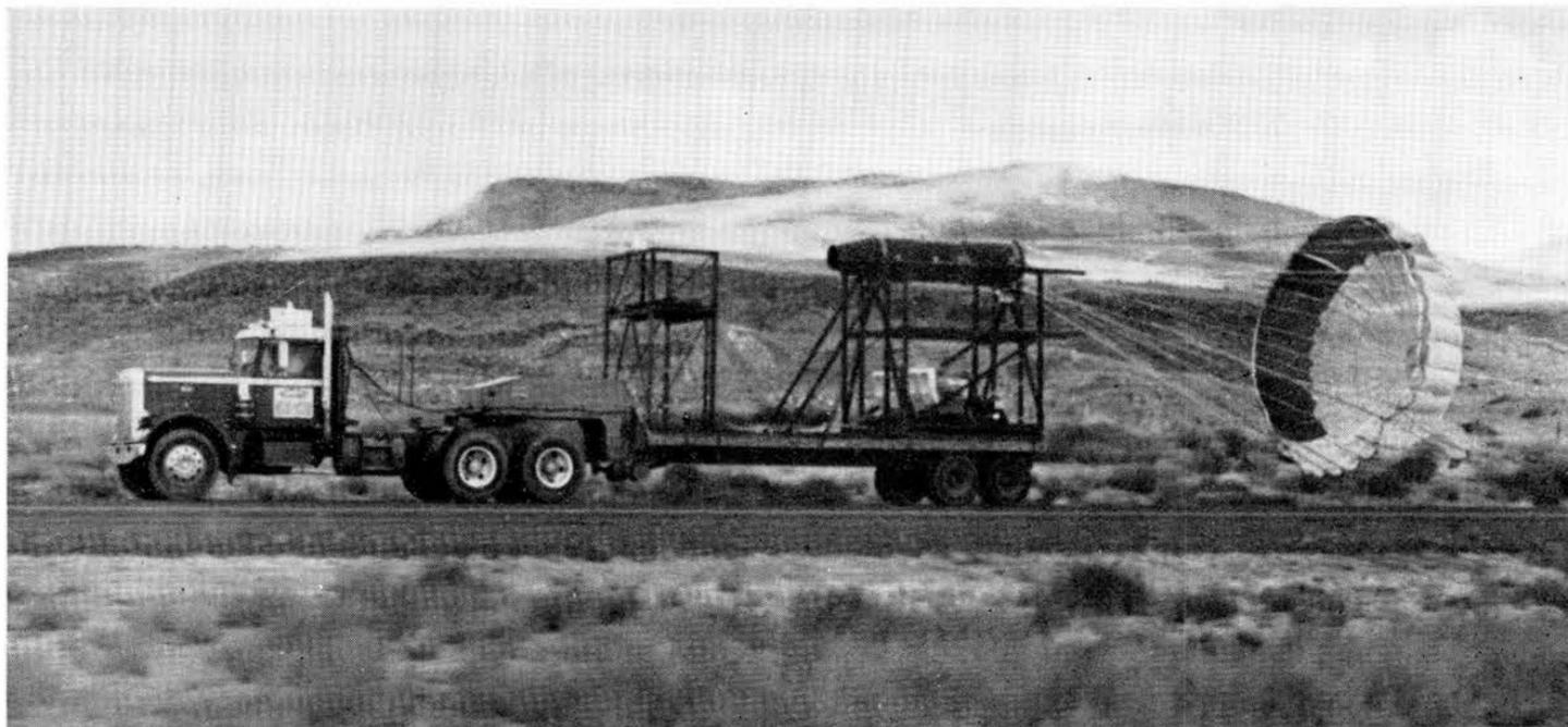
FLYING LOW—Stability tests for the chute were conducted aboard this truck on a stretch of unused freeway near Los Lunas. The oper-
